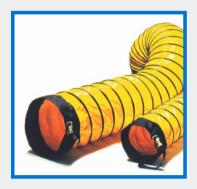
DUCT WITH QUICK CONNECT - Available in 25 or 15 foot sizes for any model. Our duct hoses are made of flexible, light duty, vinyl, woven polyester. Ducts are easily retractable and designed to handle large volumes of air at relatively low pressure. The ducts are flame retardant and easily connect to fan lips for positive and/or negative airflow. Model 1225-SC duct is dipped in static conductive material for safe use in hazardous environments.
