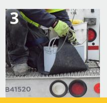
Attach Battery sling to the carabiner clip on the end of the winch line and place battery on the shelf to raise.
