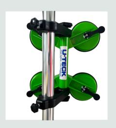
Heavy Duty Mount has secure pole fixture and clips that tighten to produce suction, then flip open to release suction. Lightweight yet strong ABS construction. Cups have 4 1/2 in diameter. total dimensions are 12 1/2 x 11in.
