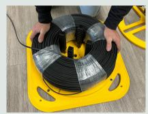
Lower cable onto coil stops.
