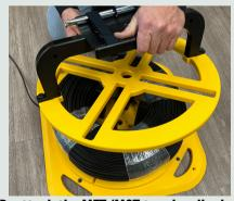
Reattach the MFT/MST tray by aligning the tray over the stops. The tray rides onto the cable and adds pressure to the coil as the coil is unwound.
