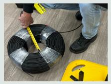
Determine the Internal Diameter by measuring the coil.
