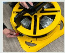
Remove the bindings once you are ready to unwind the coil.
