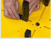
Adjust the 4 coil stops by loosening the knobs, sliding the stops inwards or outwards and adjusting them to the proper ID by aligning the arrow on each stop to the corresponding circular diameter guide.
