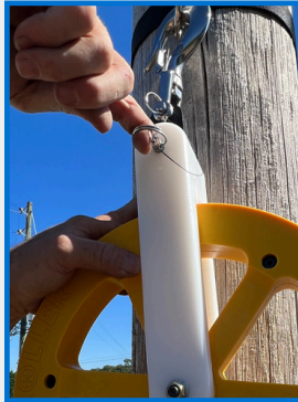
Remove retainer pin
